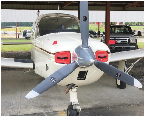
Beech Sierra Engine Inlet Plugs
