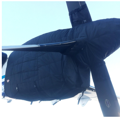
ATR-72-202 Insulated Engine & Prop Hub Covers
