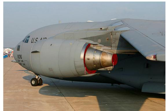
C-17 Bypass and Exhaust Plugs (illustration)
