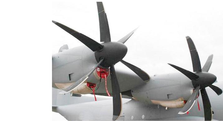
Lockheed C-130 Flight Deck Inlet/Exhaust Plugs
