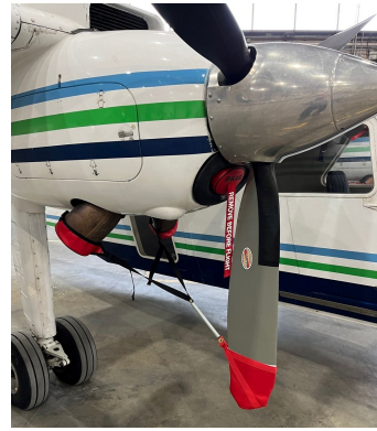
Britten-Norman Islander Engine Inlet Plugs & Prop Tie
