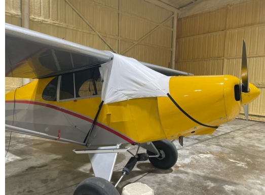
Piper J5A Windshield/Skylight Cover, test fit
