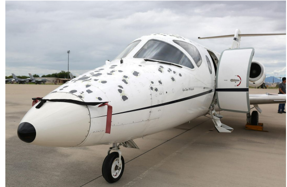
Raytheon Beechjet Hail Damage, and Pitot Covers
