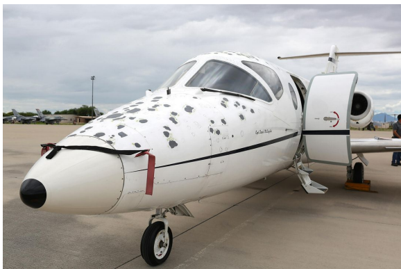
Raytheon Beechjet Hail Damage, and Pitot Covers
