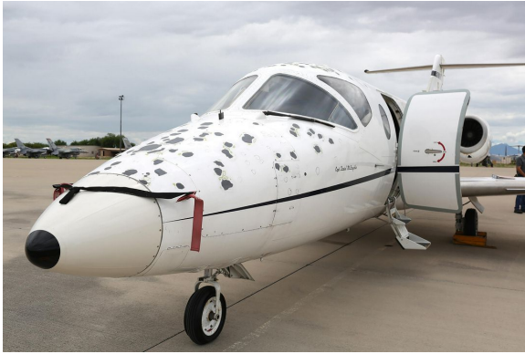
Raytheon Beechjet Hail Damage, and Pitot Covers
