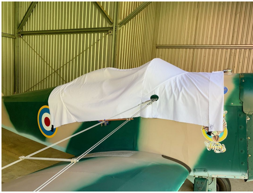
Bowers Flybaby Canopy Cover, test fit design
