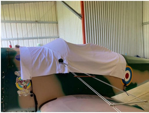
Bowers Flybaby Canopy Cover, test fit design
