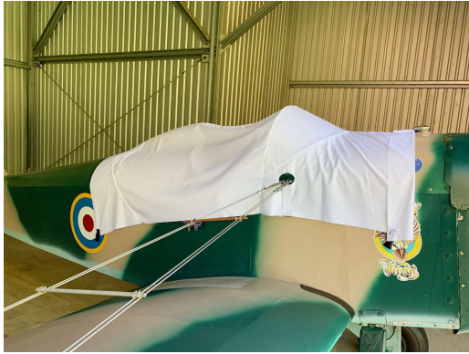
Bowers Flybaby Canopy Cover, test fit design
