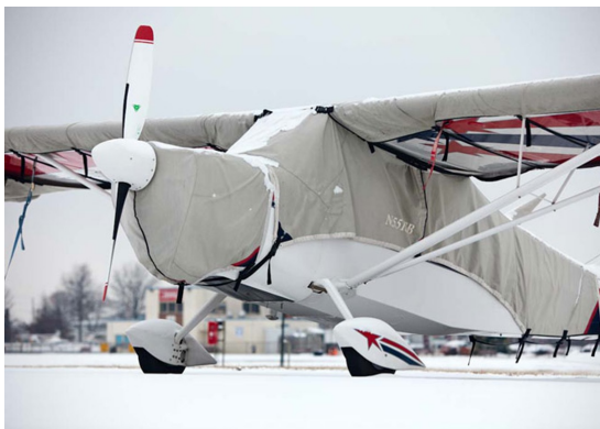
Bellanca Decathlon Canopy Cover (extended aft), Engine & Wing Covers
