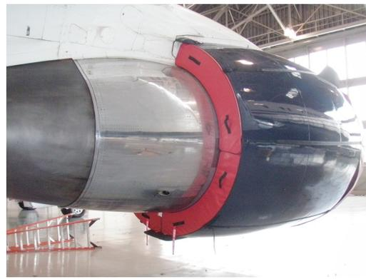
Boeing 767 Exhaust Plugs Ship Set, incl. Fan Thrust Reverser and Exhaust Plugs
