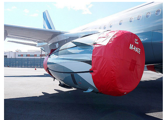
Airbus A319 Intake/Exhaust Covers set, IAE V2500
