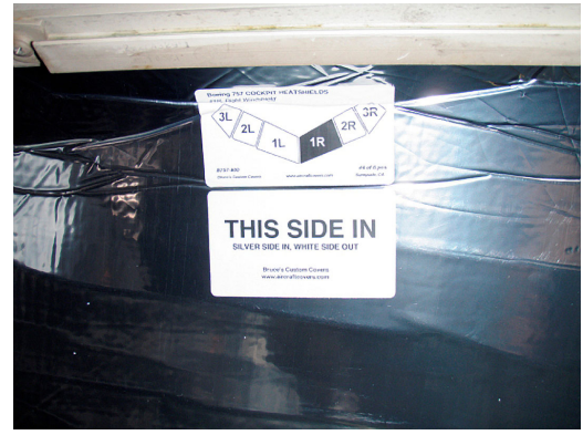
Boeing 757 Cockpit HeatShield set, installation detail
