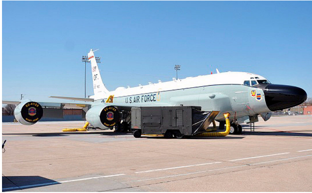
KC-135 "Tambourine" style, Double Fold Intake Covers at Offutt AFB
