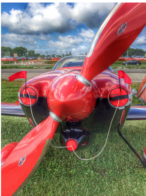
Van's RV-7 Engine Inlet Plugs
