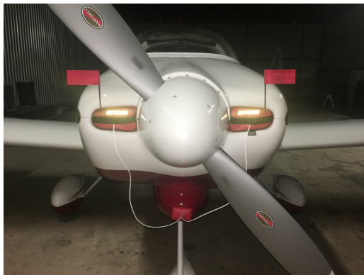
Van's Aircraft RV-7A Engine Inlet Plugs
