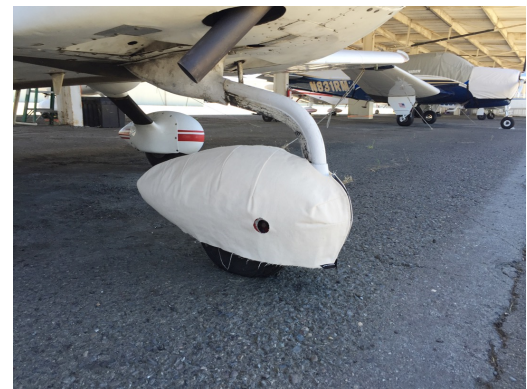
Grumman AA5 Nose Wheelpant Cover, test fit
