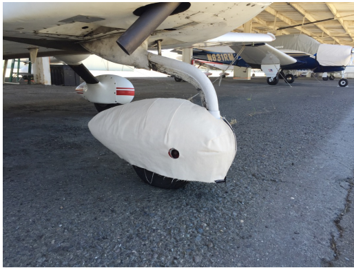
Grumman AA5 Nose Wheelpant Cover, test fit
