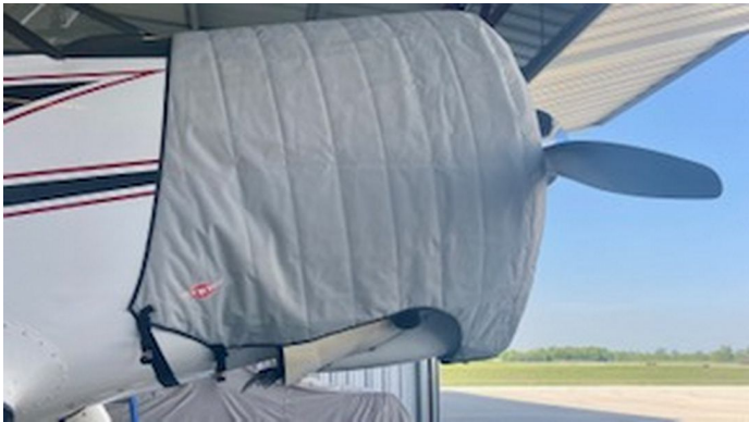
Stinson Reliant V-77, SR, AT-19 Insulated Engine Cover
