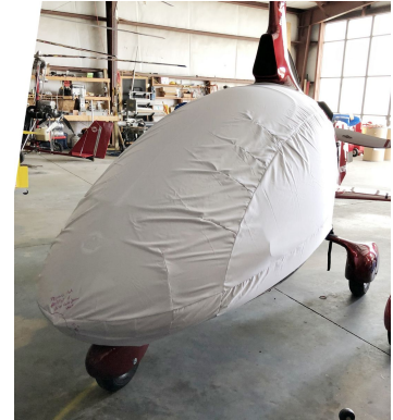
Cavalon Gyrocopter Bubble Cover, test fit cover
