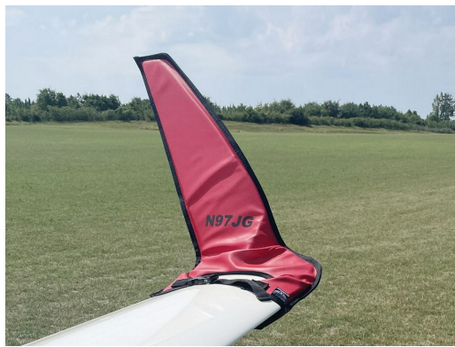
Schempp-Hirth Ventus-2B winglet/wingtip pads
