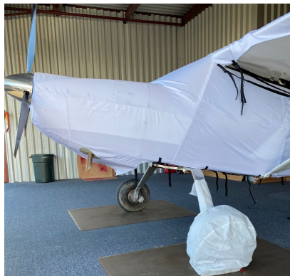
Kitfox Extended Canopy/Engine Cover, test fit cover
