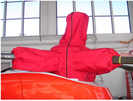
MH-65C Rotor Hub Cover w/ OADS Tube Cover detail
