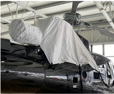
AS350 Intake/Exhaust Cover, test fit cover
