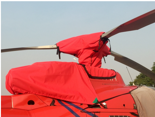
Airbus H-125 & Aerospatiale AS350 Intake/Exhaust Cover, Main Rotor Hub Cover with Weighted Skirt
