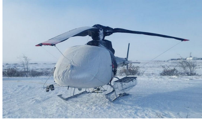
Airbus Helicopter AS350 Bubble Cover, Blade Tie-Downs, Blade Covers & Rotor Head Cover
