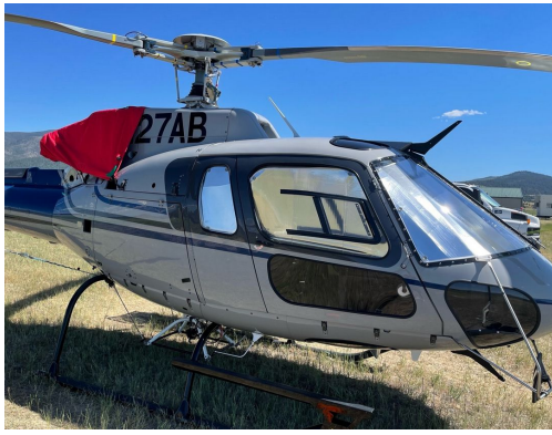
Eurocopter AS350-B3 Cabin HeatShields, Intake/Exhaust Cover
