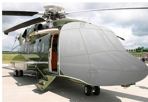
Sikorsky S-92 Windshield/Nose Cover (illustration)
