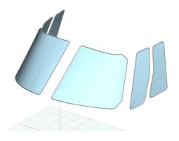
Airbus AH175 Cockpit HeatShields, 3D model
