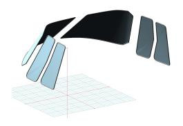
Airbus AH175 Cockpit HeatShields, 3D model
