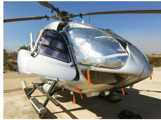
Eurocopter EC-145 Cockpit Heatshields
