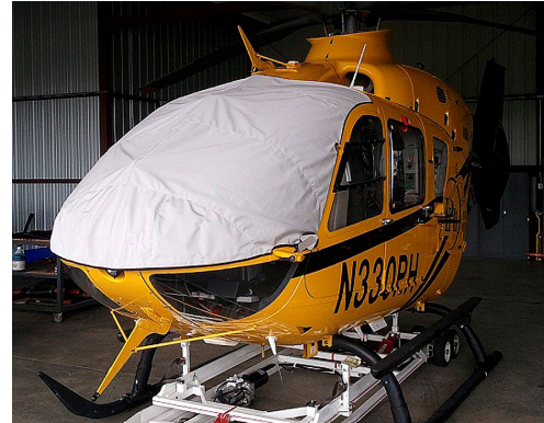
EC-135 Windshield/Skylights Cover, pinches in door jambs
