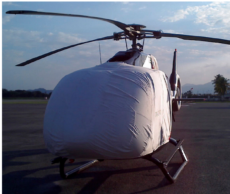
Bubble Cover and Intake/Exhaust Cover
