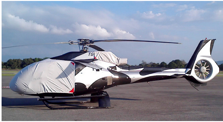
Bubble Cover and Intake/Exhaust Cover
