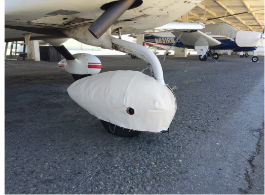
Grumman AA5 Nose Wheelpant Cover, test fit
