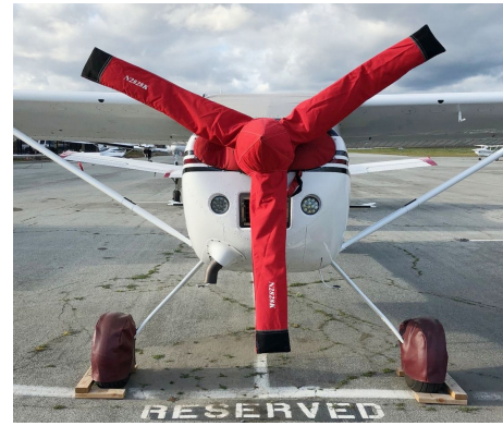
Cessna Skywagon Propellor/Spinner Cover, 3-blade type
