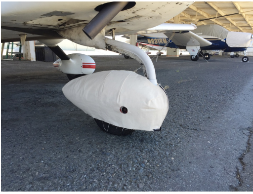
Grumman AA5 Nose Wheelpant Cover, test fit
