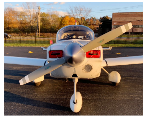
Grumman AA-5 Engine Inlet Plugs
