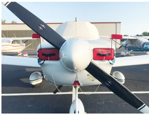
Grumman AA-5A Engine Inlet Plugs, Traveler models w/carb inlet plug (set of 3) on a
