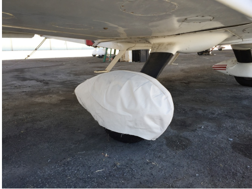
Grumman AA5 Main Wheelpant Cover, test fit
