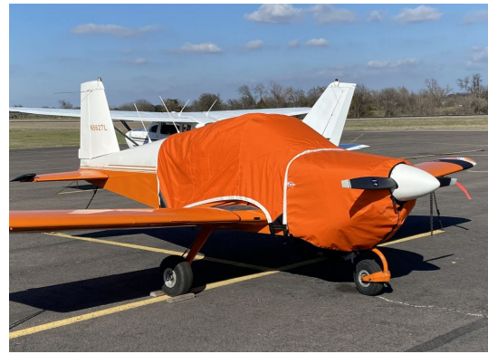
AA-1 Extended Canopy & Fully Enclosed Engine Cover
