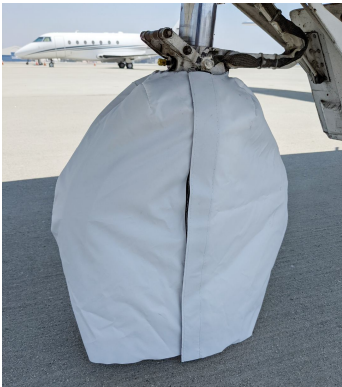
CJ1 Nose Gear Tire Cover, test fit
