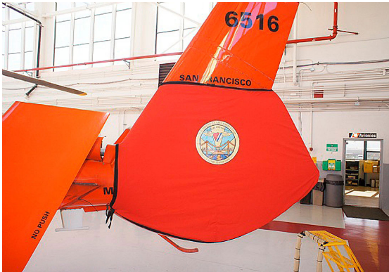
MH-365C Dauphin Tail Fan Fenestron Cover
