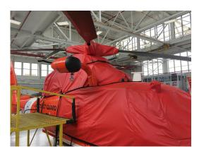
MH-65C Bubble Cover, extended Nose/Radome Model, padded over U.S. Coast Guard HH-65 Dolphin Bubble, Engine & Rotor windows, P/N: A365-210 Mast Covers
