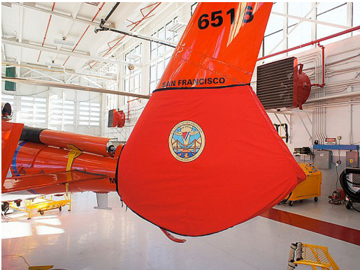
MH-365C Dauphin Tail Fan Fenestron Cover
