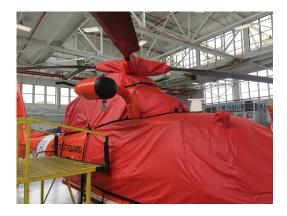
MH-65C Bubble Cover, extended Nose/Radome Model, padded over U.S. Coast Guard HH-65 Dolphin Bubble, Engine & Rotor windows, P/N: A365-210 Mast Covers
