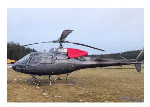
Airbus Helicopter AS350 Intake/Exhaust Cover
