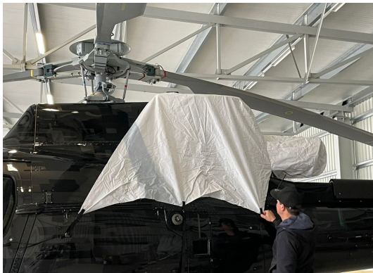
AS350 Intake/Exhaust Cover, test fit cover
