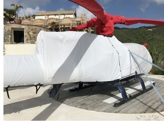
Aerospatiale Gazelle AS341 Bubble, Rotor Mast, Blade, Engine & Tailboom Covers (some are test fit covers)
