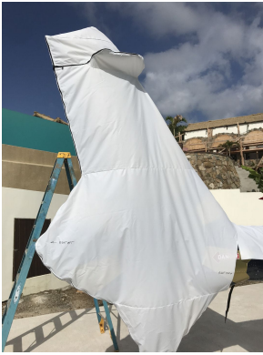
Aerospatiale Gazelle AS341 Tailfan Housing Extended Cover (test fit cover)
