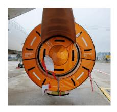
Airbus A320 Exhaust & Bypass Vent Plugs
