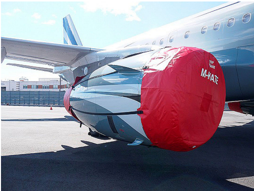
Airbus A319 Intake/Exhaust Covers set, IAE V2500
