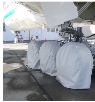
Boeing 777 Main & Nose Gear Tire Covers
