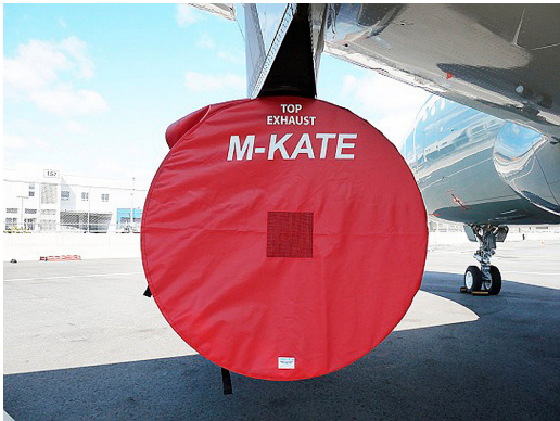
Airbus A319 Intake/Exhaust Covers set, IAE V2500
