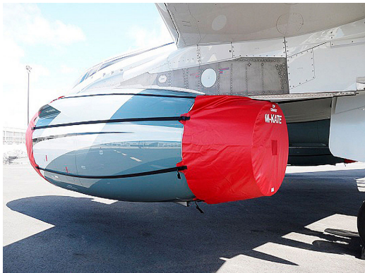
Airbus A319 Intake/Exhaust Covers set, IAE V2500
