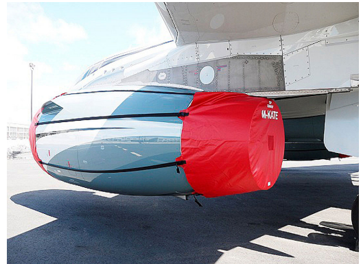
Airbus A319 Intake/Exhaust Covers set, IAE V2500 engine shown
