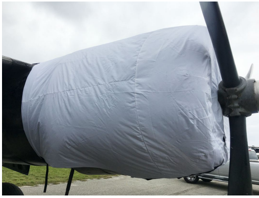
Douglas A-26 Engine Cover, test fit cover
