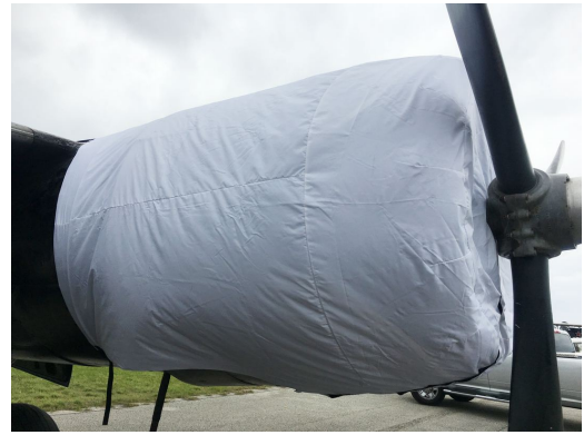
Douglas A-26 Engine Cover, test fit cover
