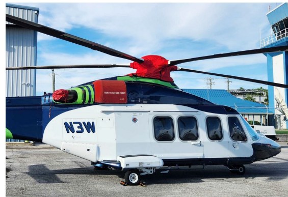
Agusta AW139 Rotor Mast Cover, covers upper deck & aft of rotor mast area
