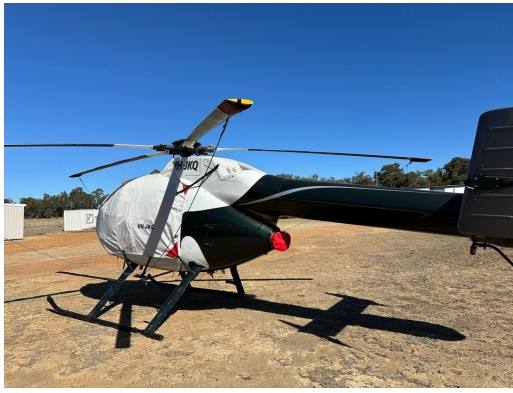
MDD 520 NOTAR Bubble Cover w/Intake Cover Add-On, Exhaust Cover MH-6J Bubble, Flir & Doghouse Covers (illustration)
