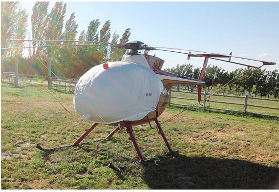
MD500D Bubble Cover with Intake Add-On
