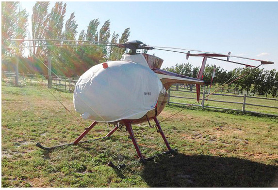
MD500D Bubble Cover with Intake Add-On
