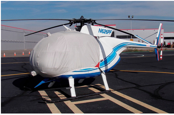
MD500C Bubble Cover with Wire Strike detail
