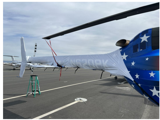
Bell 505 Tailboom & Stabilizer Covers, test fit cover
