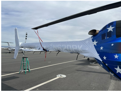
Bell 505 Tailboom & Stabilizer Covers, test fit cover
