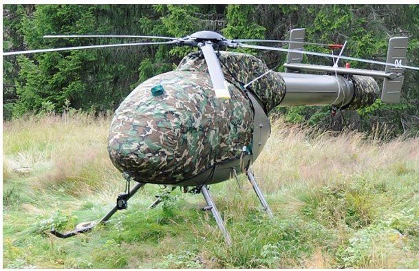
MD520 NOTAR Bubble, Engine, & NOTAR Covers & Blade Tie-downs Hughes 500D Bubble Cover with Wire Strike detail and Blade Tie-downs
