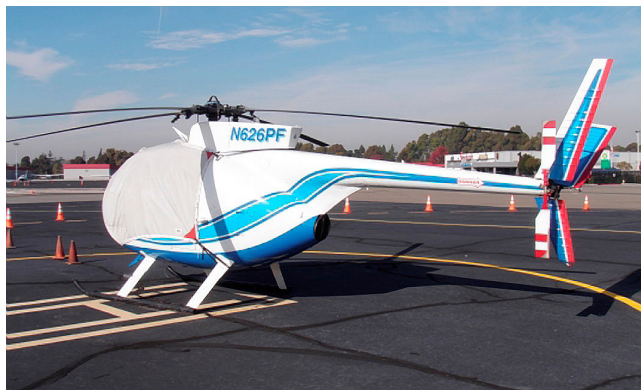
MD500C Bubble Cover with Wire Strike detail
