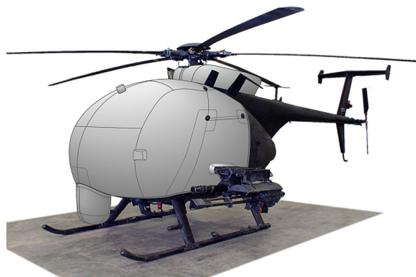
MH-6J Bubble, Flir & Doghouse Covers (illustration)
