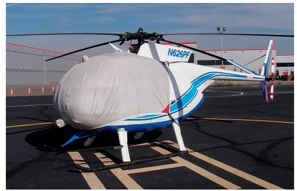
MD500C Bubble Cover with Wire Strike detail
