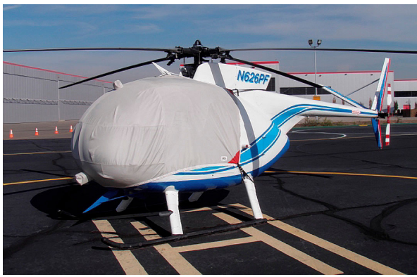
MD500C Bubble Cover with Wire Strike detail
