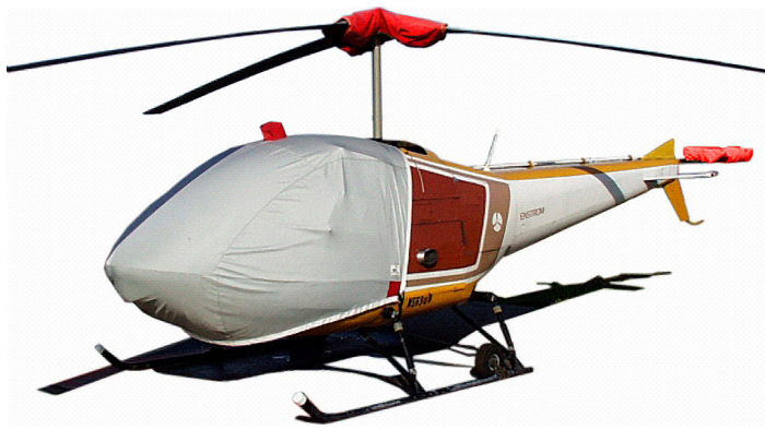
Enstrom 280FX Bubble, Main Rotor Mast, Tail Rotor Covers on Enstrom F280FX
