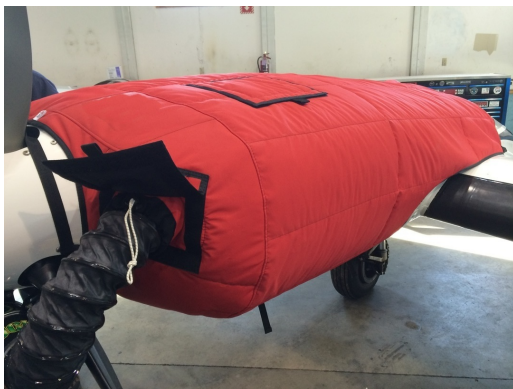
Cessna 402 Insulated Engine Cover with Heater
