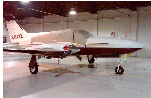
Cessna 414 Canopy Cover and Engine Inlet Plugs
