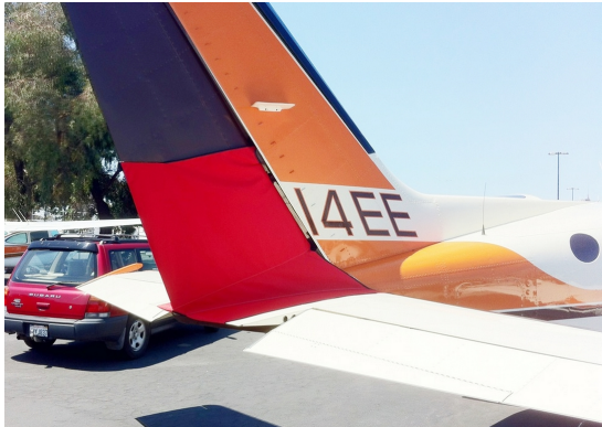
Cessna 414 Rudder Openings Cover (bird barrier)
