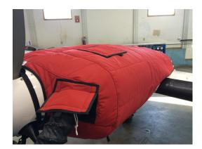
Cessna 402 Insulated Engine Cover with Heater
