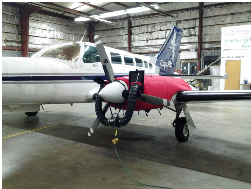
Cessna 402 Insulated Engine Cover with Heater
