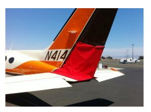
Cessna 414 Rudder Openings Cover (bird barrier)
