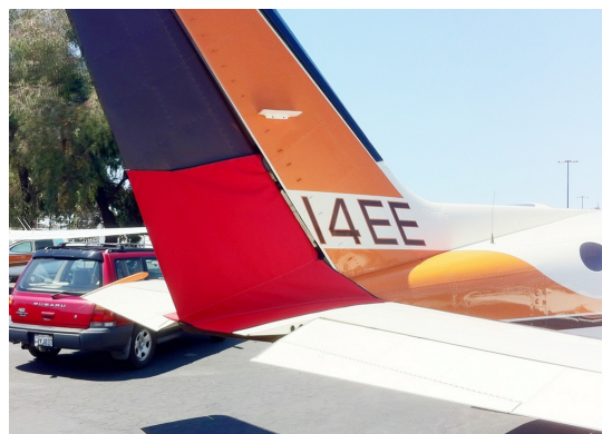
Cessna 414 Rudder Openings Cover (bird barrier)
