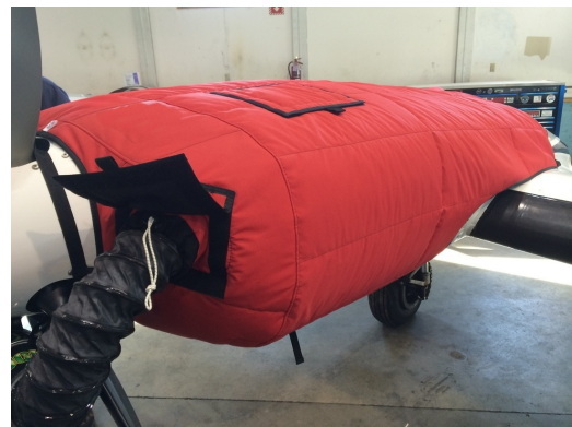
Cessna 402 Insulated Engine Cover with Heater
