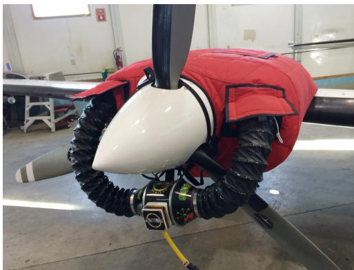
Cessna 402 Insulated Engine Cover with Heater
