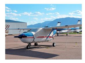
Cessna Sky Master Canopy Cover, extended down to cover Cessna 337 Skymaster Canopy Cover, Forward Engine Plugs and door.
