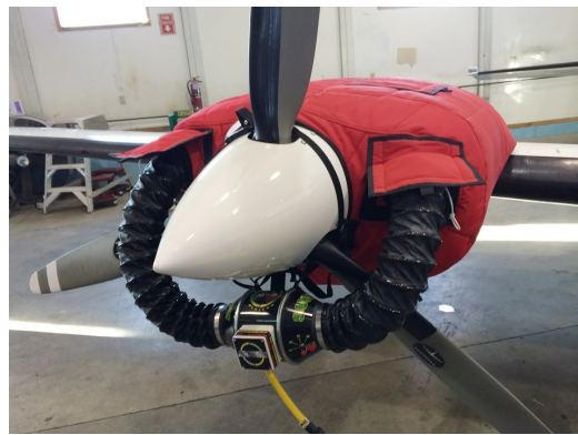
Cessna 402 Insulated Engine Cover with Heater
