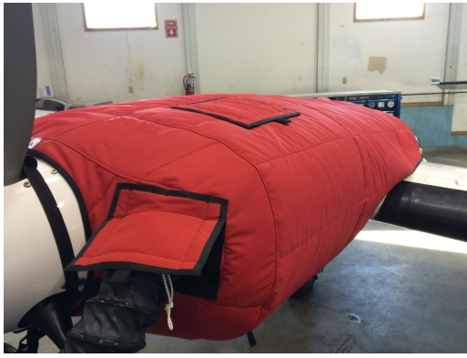
Cessna 402 Insulated Engine Cover with Heater
