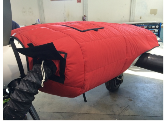
Cessna 402 Insulated Engine Cover with Heater
