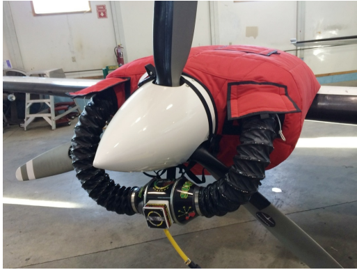
Cessna 402 Insulated Engine Cover with Heater
