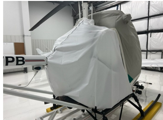
Schweizer 300C Engine Cover, test fit cover
