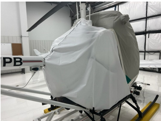
Schweizer 300C Engine Cover, test fit cover
