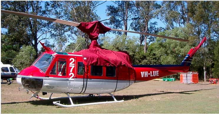
Bell 204/205 Engine/Mid-Cabin Cover, Main & Tail Rotor Covers
