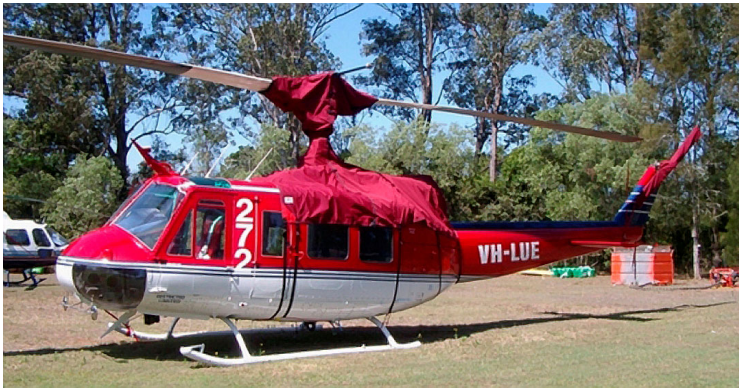
Bell 204/205 Engine/Mid-Cabin Cover, Main & Tail Rotor Covers
