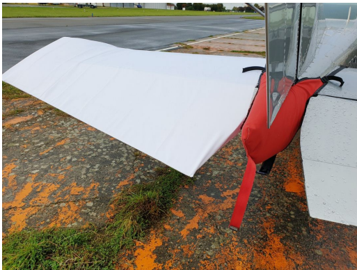
Cessna 207 Tailcone Cover, Horizontal Stab. Cover (test fit)
