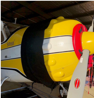
Cessna 195 Engine Plugs, Cowl Ring Gap Cover
